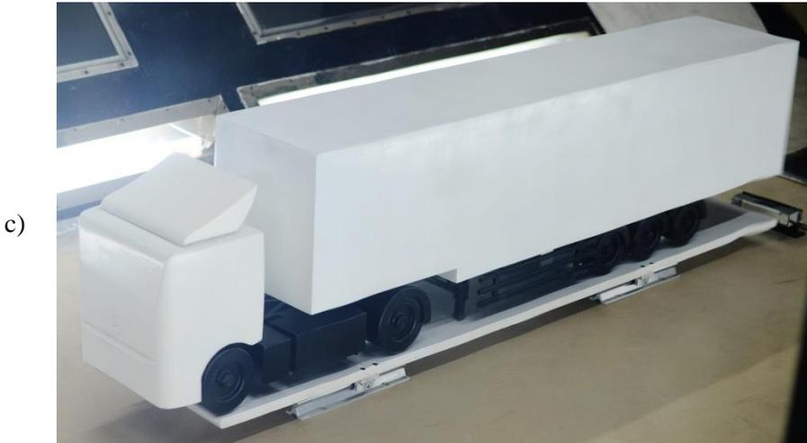
Figure 6. Testing models by three configurations in the wind tunnel
