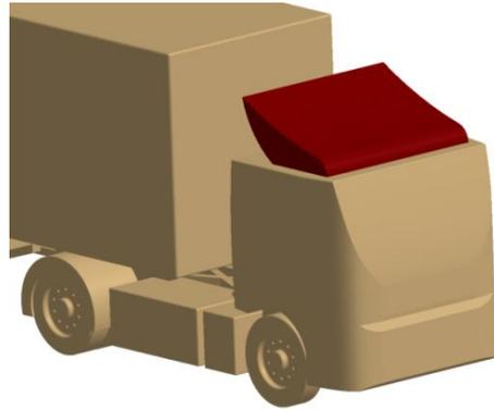
*Figure 4. Optimized spoiler on the top of the truck cab*
