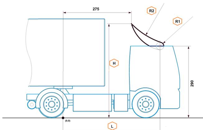
Figure 3. Initial position of the spoiler with parameters
