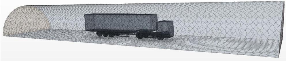
Figure 2. CFD mesh view of the testing model
